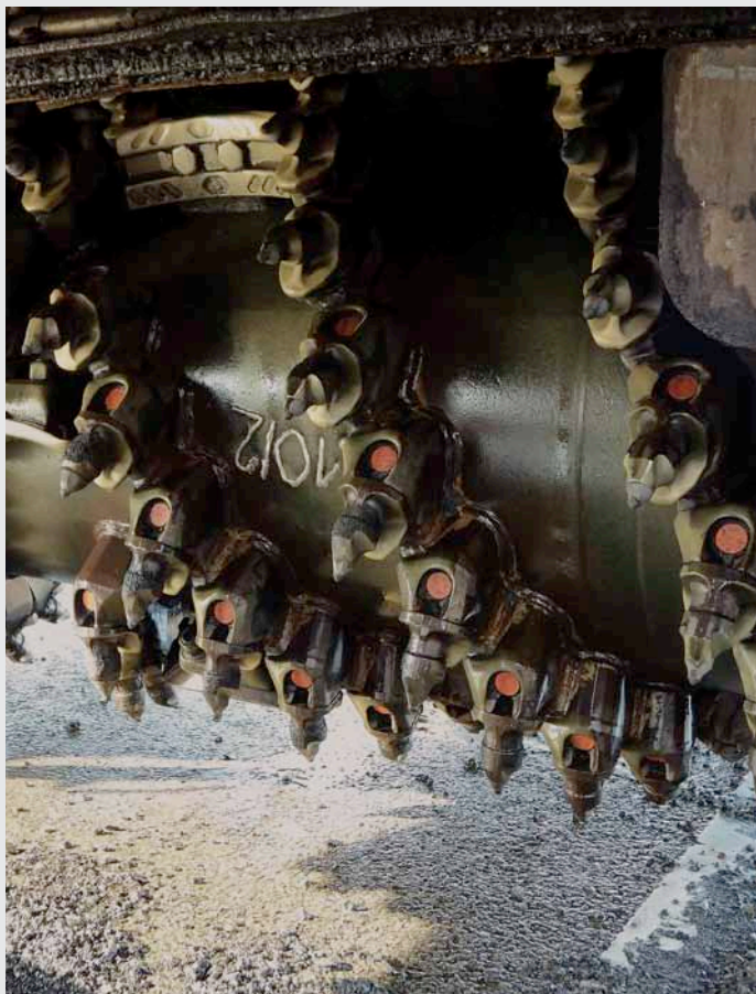
Element Six D Power™ Road Picks last in excess of 40 times longer than standard picks.
